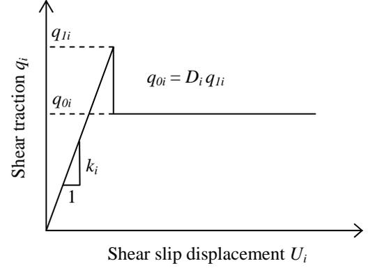
Figure 2: Mechanical behavior of infill material.
