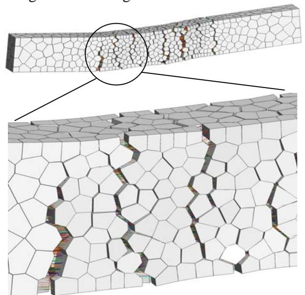
**Figure 4:** Multiple crack formation within lattice model
