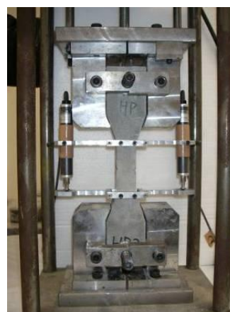
Photo 1: Uniaxial tension testing apparatus
