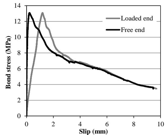
**Figure 8:** Bond stress versus slip behaviour: RSF concrete (RB\_2)
