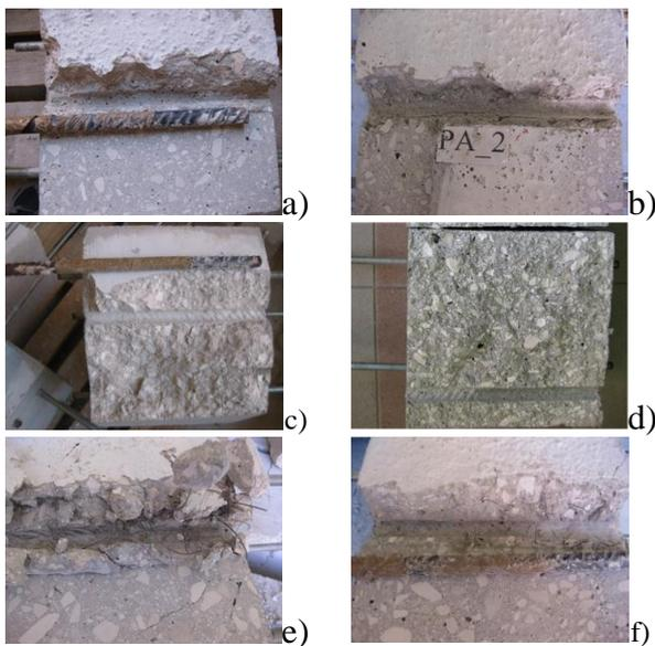
**Figure 6:** Bonding interface between steel rebar and concrete matrix for the specimens: a)PA1; b)PA2; c) PB2; d)PC1; e)RA3; f)IB3
