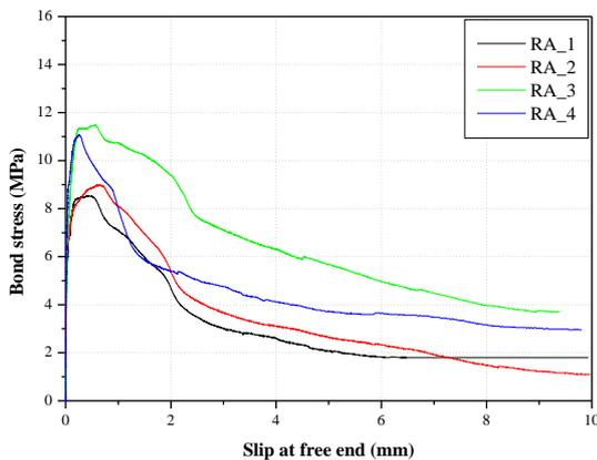
**Figure 9:** Bond stress versus free end slip for RSFRC - configuration "A"
