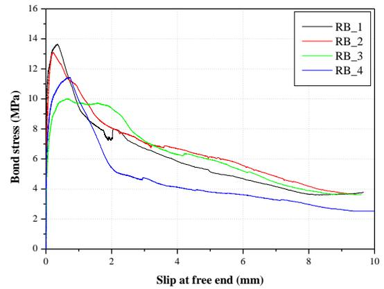
**Figure 10:** Bond stress versus free end slip for RSFRC - configuration "B"
