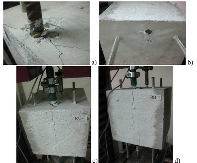
**Figure 13:** Failure of specimens realized with RSF: a) loaded end of RA\_1; b) free end of RB\_2; c) overall view of RC\_1; d) overall view of RB\_1.
