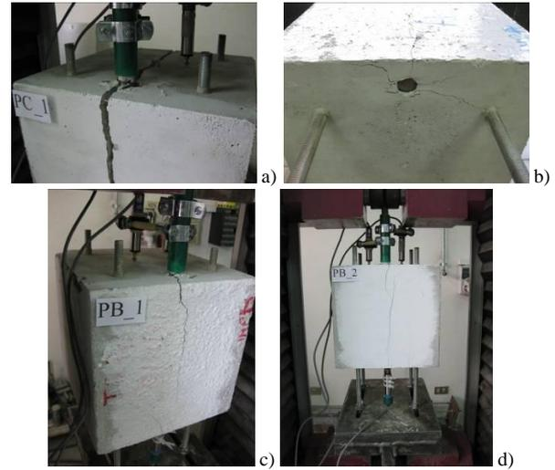
**Figure 12:** Failure of specimens realized with plain concrete: a) loaded end of PC\_1; b) free end of PA\_1; c) overall view of PB\_1; d) overall view of PB\_2
