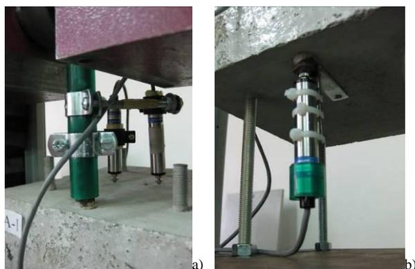
**Figure 4:** Positions of the displacement transducers: a) loaded end, b) free end
