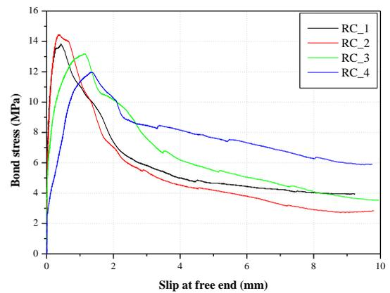
**Figure 11:** Bond stress versus free end slip for RSFRC - configuration "C"
