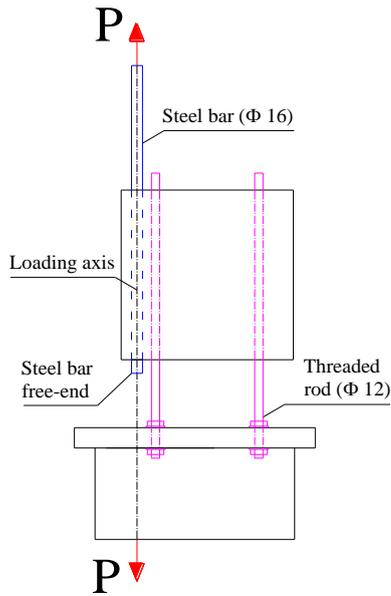
Figure 1: Bond test set-up.
