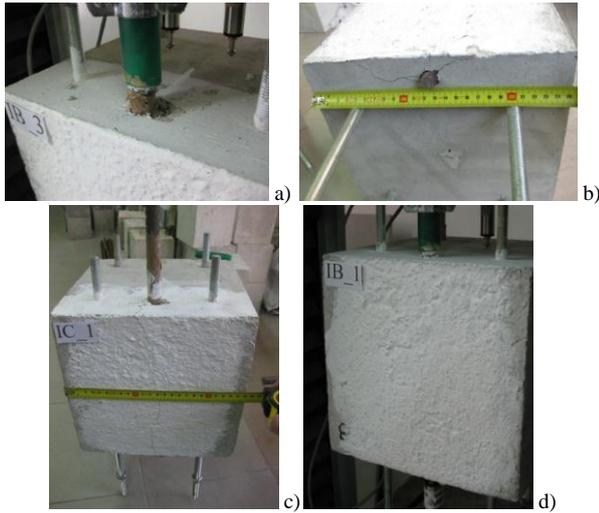
**Figure 14:** Failure of specimens realized with ISF: a) loaded end of IB\_3; b) free end of IA\_1; c) overall view of IC\_1; d) overall view of IB\_1.
