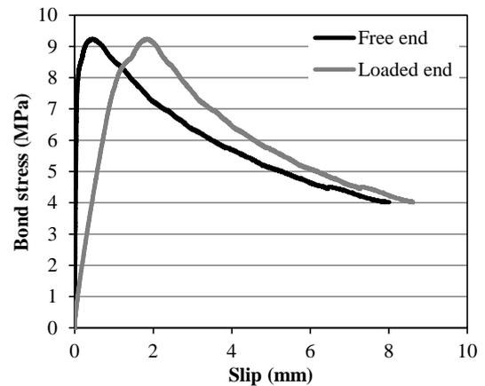
**Figure 7:** Bond stress versus slip behaviour: plain concrete (PA\_1)
