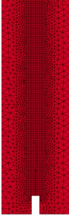
Figure 8: Macroscopic model – Mesh of the DCB specimen.
