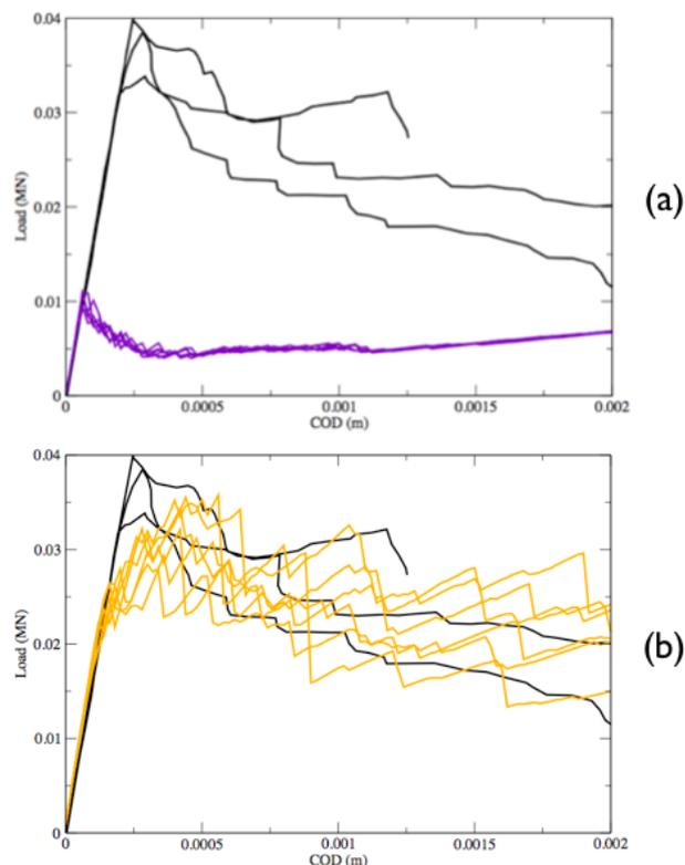
Figure 7: Results obtained with the discrete model – same mesh as in Figure 3 – and the use of linear contact elements: (a) local elastic-brittle behaviour, (b) cohesive-crack approach. Experiments are in black.
