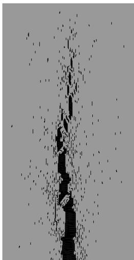
Figure 6: Example of crack pattern obtained with the discrete model on a refined mesh (zoom on the crack tip).
