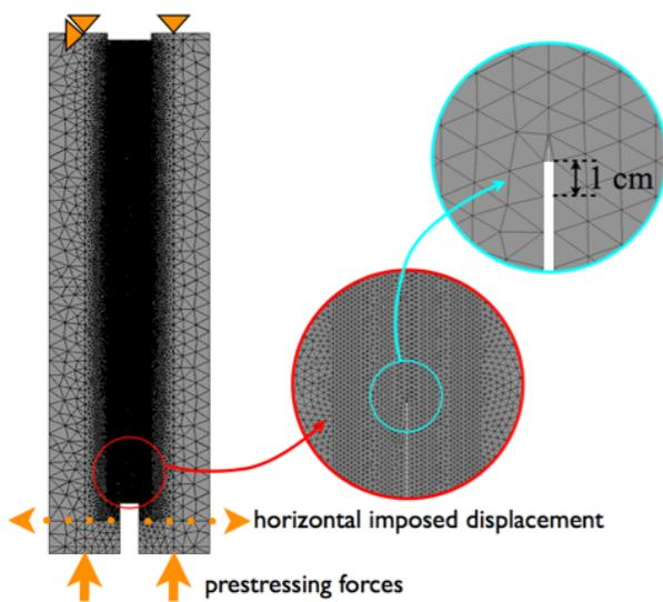
Figure 3: Discrete model – Mesh, boundary and loading conditions.
