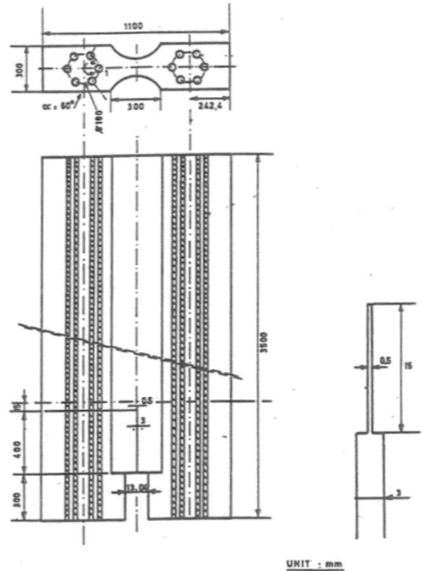
**Figure 1:** Geometry of the DCB specimen.
