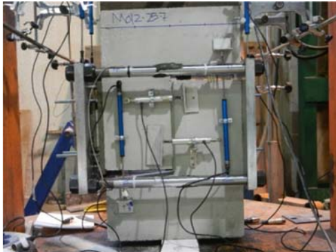
Figure 7: Disposition of the LVDT's and strain gages
