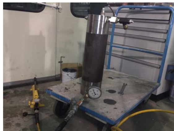
Figure 4: Pressure accumulator device for constant pressure.
