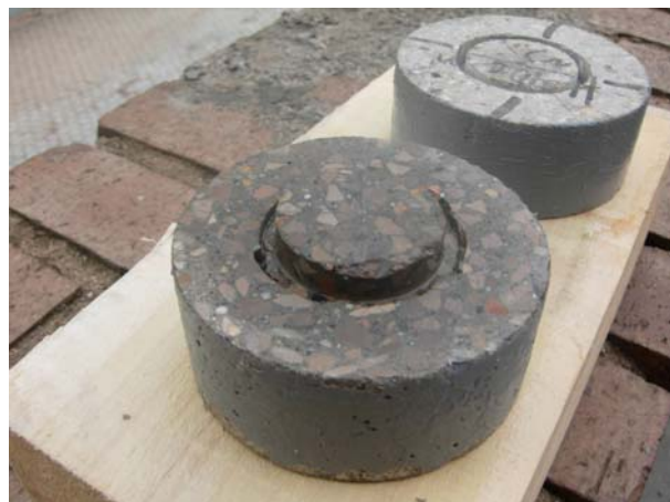
Figure 7: Radial cracks in a specimen tested under confining pressure of 8 MPa.
