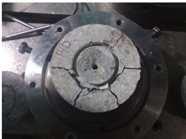
Figure 6: State of specimen after the unconfined test, with large fully developed radial cracks.
