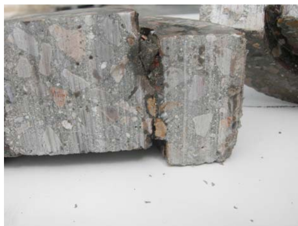
Figure 8: Fracture plane observed in tested specimen, at bottom end observe the displaced aggregate which has been cut through in two pieces by a sensibly straight crack.
