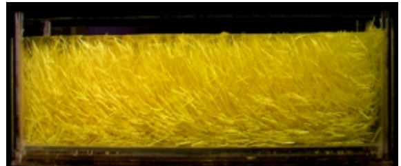
Figure 8: Fiber orientation of PVA fiber (3.0%)
