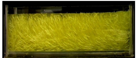
Figure 7: Fiber orientation of PVA fiber (2.0%)
