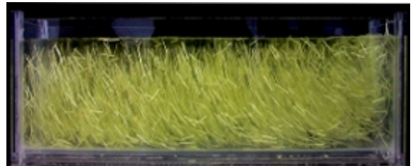
Figure 6: Fiber orientation of PVA fiber (1.0%)
