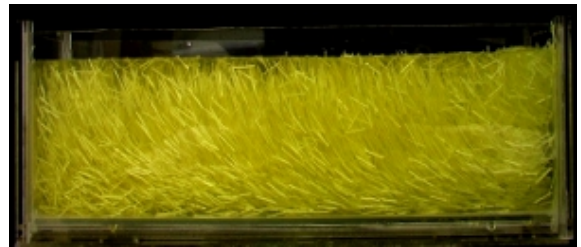
Figure 7: Fiber orientation of PVA fiber (2.0%)
