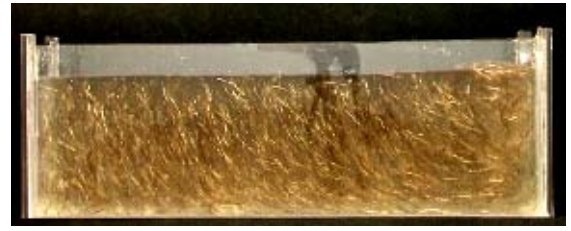
Figure 5: Fiber orientation of steel fiber (0.5%) by flow-filling
