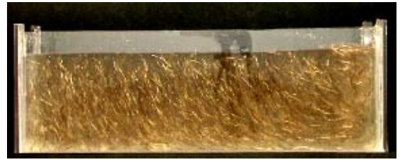
Figure 5: Fiber orientation of steel fiber (0.5%) by flow-filling
