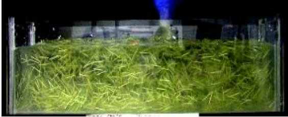
Figure 9: Fiber orientation of PVA fiber (0.5%) by move-filling
