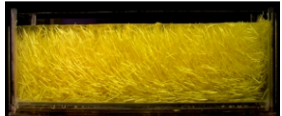
Figure 8: Fiber orientation of PVA fiber (3.0%)
