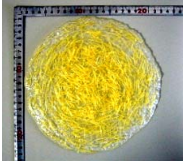
Figure 3: Flow of visualization model concrete
