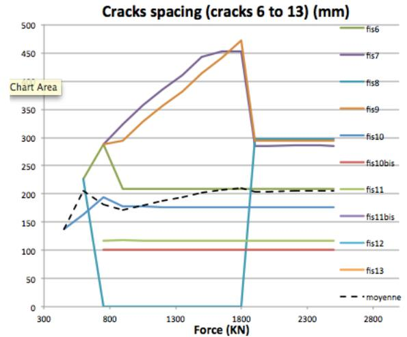
**Figure 17:** Cracks spacing estimated by experimental data from digital image correlation, for a 2500 kN loading along 1800 mm in the central part of the beam.
