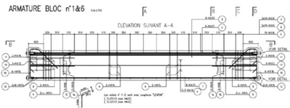
Figure 2: Layout of reinforced of the beam.
