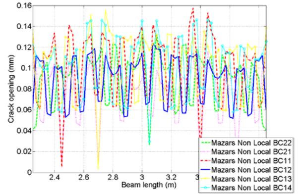
**Figure 14:** Cracks opening according to Mazars model along the horizontal top line (at  $y = 800$  mm).
