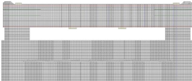
**Figure 6:** Finite element mesh used in the second modelling. Concrete is represented in black, steel reinforcement bars in red and green, U and stirrups in blue, macalloy steel rebars in violet and the loading and support platens in yellow.
