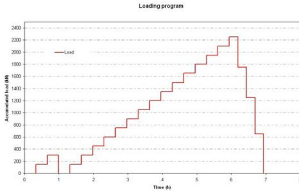
Figure 4: Monotonic loading applied on the beam.
