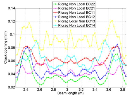
**Figure 15:** Cracks opening according to Ricrag model along the horizontal top line (at  $y = 800$  mm).
