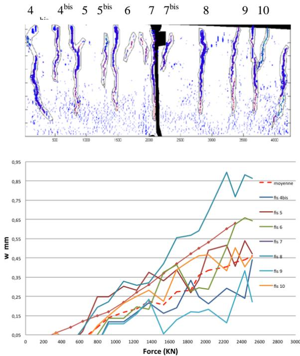
**Figure 16:** Experimental crack distribution (crack openings) for a 2500 kN loading along 1800 mm in the central part of the beam, digital image correlation (DIC).
