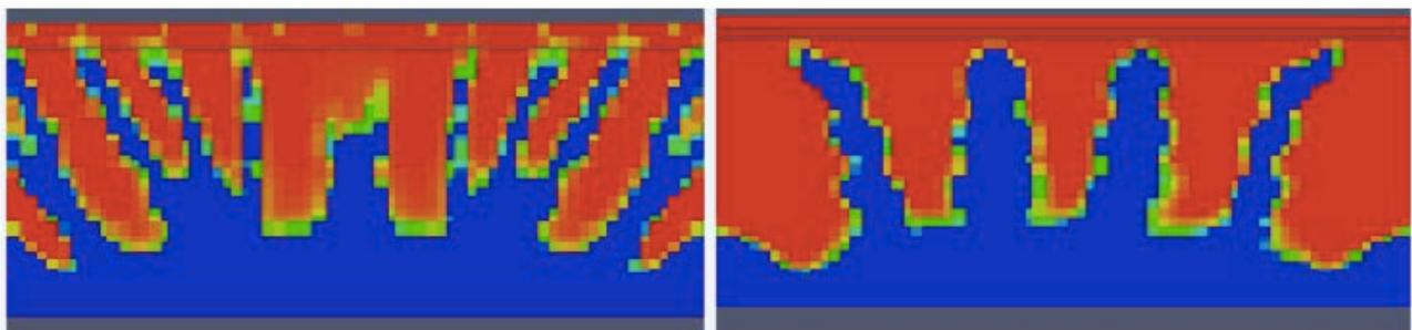
**Figure 13:** Damage patterns in the central part of the beam (1600 mm) obtained with Mazars (left) and Ricrag (right) models obtained for 14 mm mid span displacements with BC22 boundary conditions.
