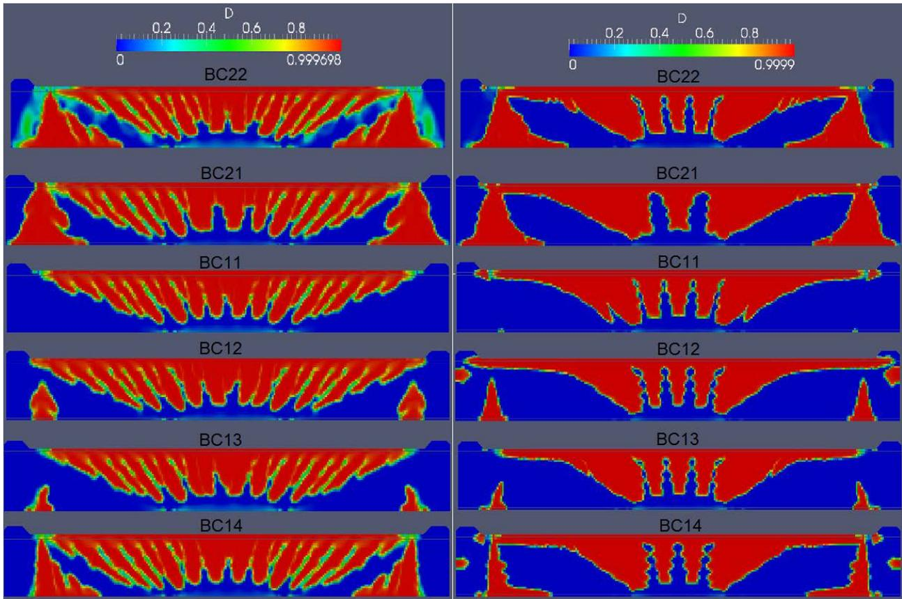
**Figure 12:** Damage pattern with Mazars and Ricrag models obtained for 14 mm mid span displacements with BC22, BC21, BC11, BC12, BC13 and BC14 boundary conditions.
