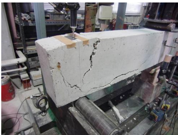
Figure 11: Splitting at the beam ends (SG, Series 0 with hooks)
