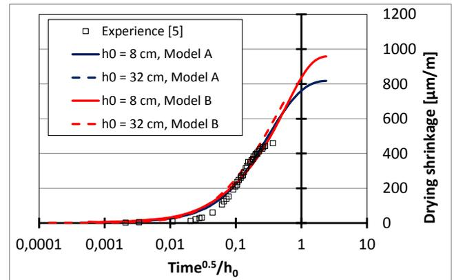
**Figure 4:** Evolution of drying shrinkage, predicted by the two phenomenological models (for two volume to surface ratios:  $h_0/2$ ) with respect to the ratio between the square root of time and  $h_0$ . Models A and B corresponds to Equation 10 and 11, respectively.
