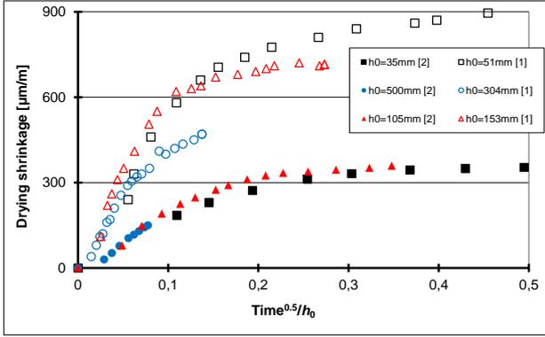
**Figure 1:** Evolution of drying shrinkage (for different volume to surface ratio:  $h_0/2$ ) with respect to the square root of time to  $h_0$  ratio [1,2]. Only partial data are displayed for sake of clarity.
