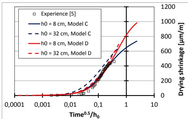
**Figure 4:** Evolution of drying shrinkage, predicted by the two phenomenological models (for two volume to surface ratios:  $h_0/2$ ) with respect to the ratio between the square root of time and  $h_0$ . Models C and D corresponds to Equation 7 and 8, respectively.
