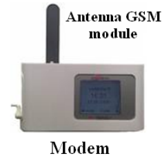
Figure 2: Central Unit interface (a). Modem for AE wireless data transmission (b).
