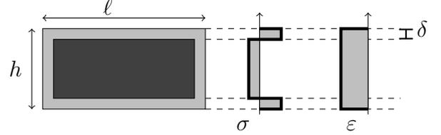
Figure 4: Stress and strain distribution in a central cross section.
