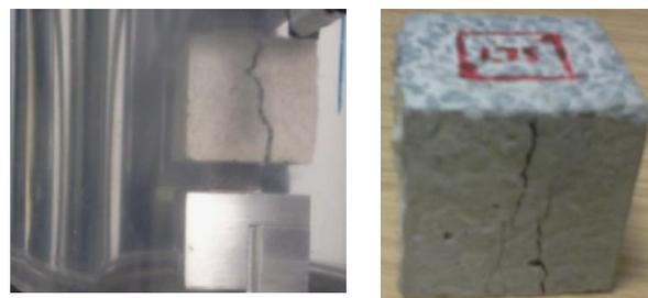
**Figure 2:** A specimen under loading and after the test
