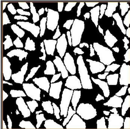
Figure 6: Segmented aggregates
