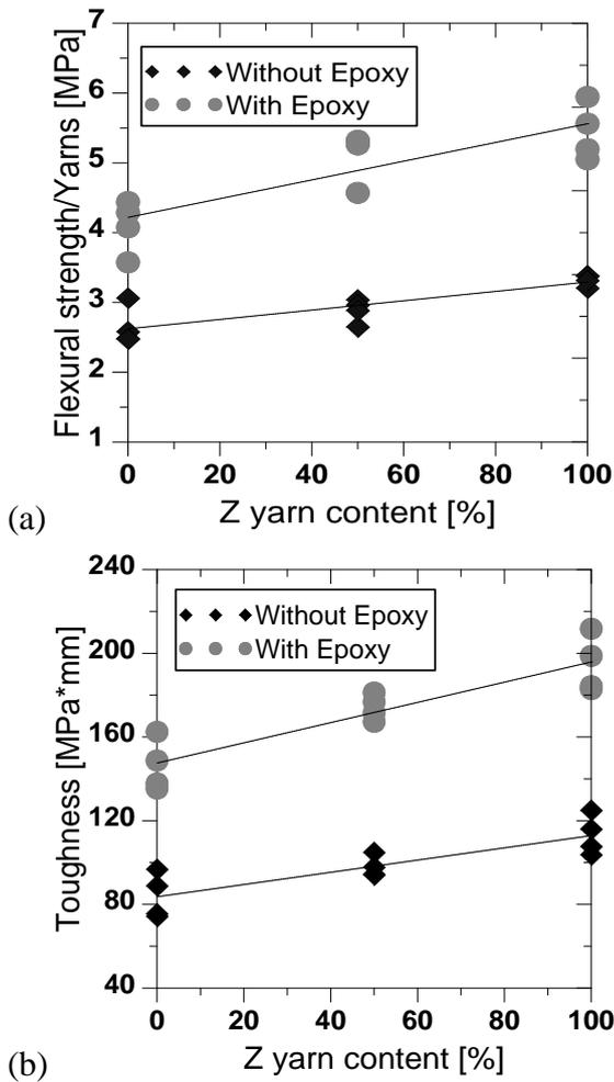
**Figure 4:** Flexural properties vs. aramid Z yarn content (a) flexural strength, (b) toughness, with and without epoxy
