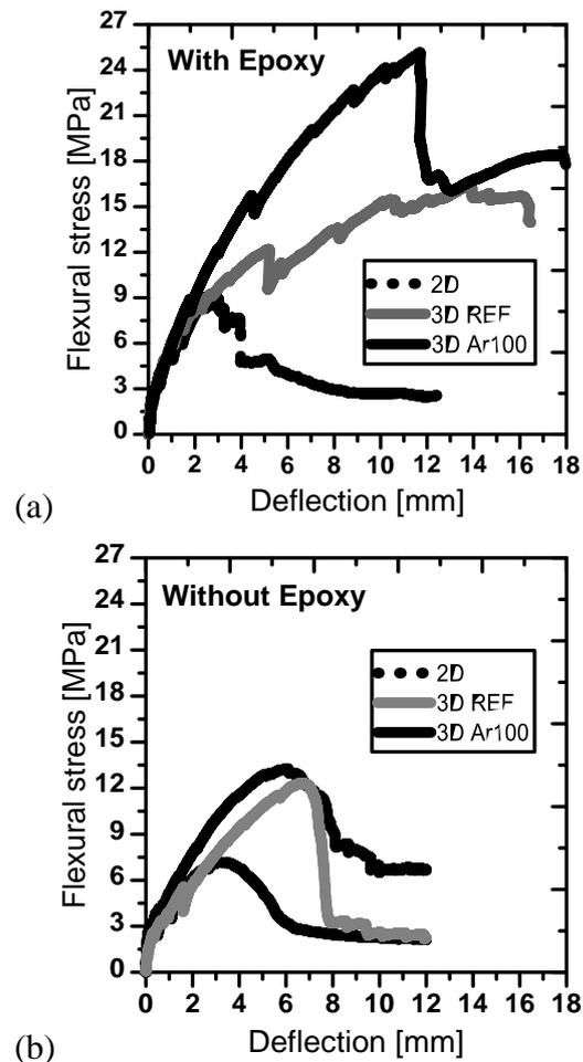
**Figure 3:** Flexural behavior of the composites with the 2D fabric, and 3D fabrics with and without (REF) aramid yarns: (a) with epoxy, (b) without epoxy.
