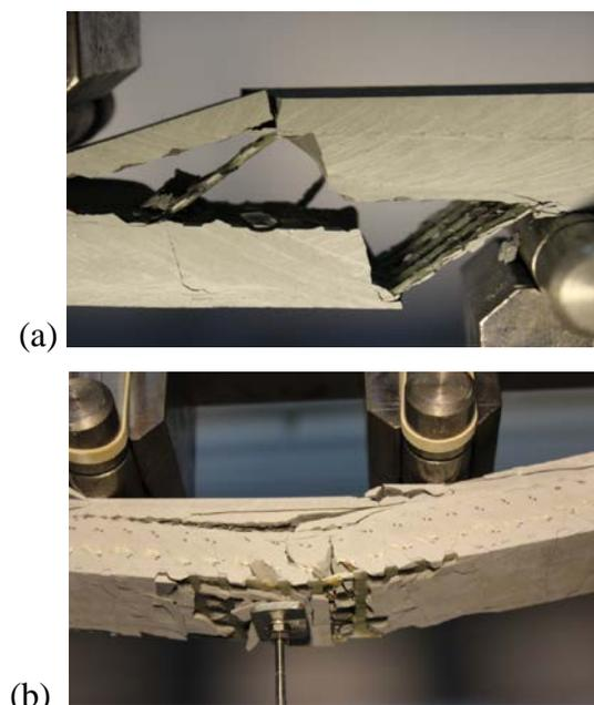
**Figure 8:** Failure mechanism of (a) 2D fabric composite and (b) 3D Ar100 composite at the end of testing.
