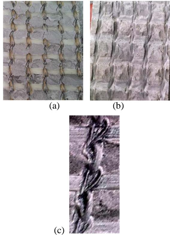
**Figure 5:** (a, b) Anchoring of the fabric within the cement matrix, a. the fabric itself, b. print of the fabric structure within the matrix, (c) anchoring of the loops in the matrix.
