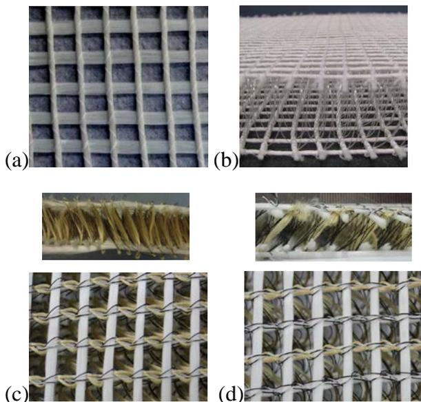
**Figure 2:** Different fabrics: (a) 2D, (b) 3D REF, (c) 3D Ar100 top and side view, and (d) 3D Ar50 top and side view
