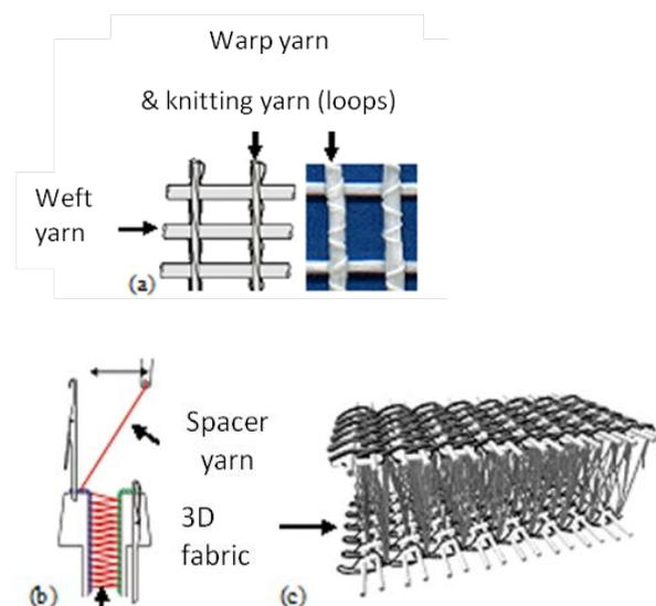
**Figure 1:** (a) 2D warp knitted fabric at both faces of the 3D fabric, (b) schematic description of the 3D fabric production, and (c) simulated 3D fabric.
