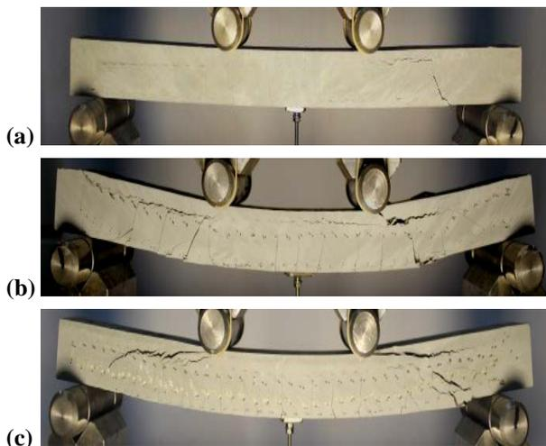
**Figure 7:** (a) 2D, (b) 3D REF and (c) 3D Ar100 composites with epoxy
