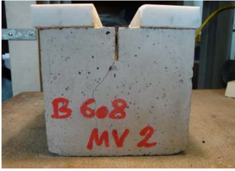
Figure 1: Concrete specimen for the wedge splitting test according to Tschegg [6, 7].
