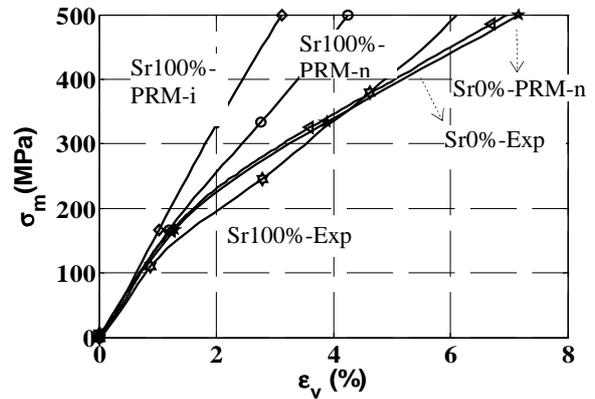
**Figure 12.** Mean stress vs. volumetric strain: Comparisons of experimental results with simulation results obtained with the initial (PRM-i) and new model (PRM-n) for saturated and dry concrete under high confinement.
