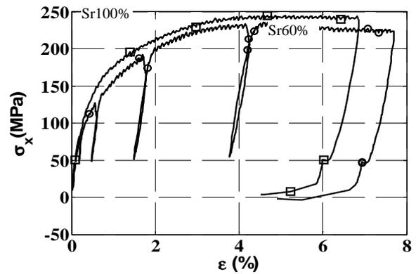
Figure 4: Comparison of axial behavior at 50 MPa of confining pressure for two different saturation ratios of concrete specimens
