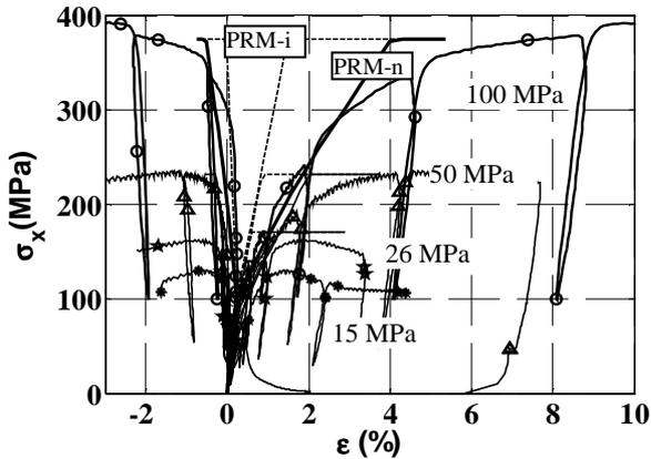
**Figure 10.** Axial stress vs. axial and circumferential strains: Comparisons of experimental results with simulation results obtained with the initial (PRM-i) and new model (PRM-n) for a wet concrete specimen under moderate confinement.
