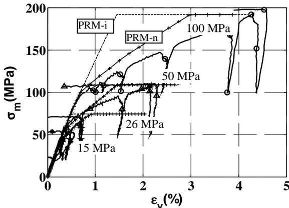
**Figure 11.** Mean stress vs. volumetric strain: Comparisons of experimental results with simulation results obtained with the initial (PRM-i) and new model (PRM-n) for a wet concrete specimen under moderate confinement.
