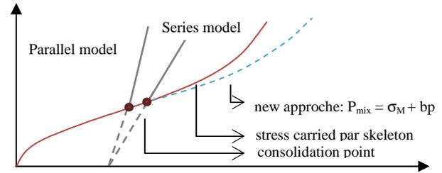
**Figure 9.** Diagram of stress calculation according to the poromechanical approach as concrete gets consolidated
