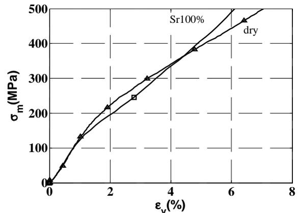
Figure 5. Hydrostatic behavior of concrete for two different degrees of saturation
