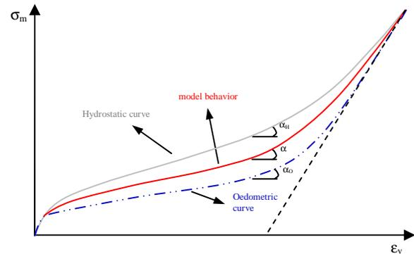
**Figure 8.** Hydrostatic behavior, oedometric behavior and consolidated behavior of concrete: mean stress in function of volumetric strain.
