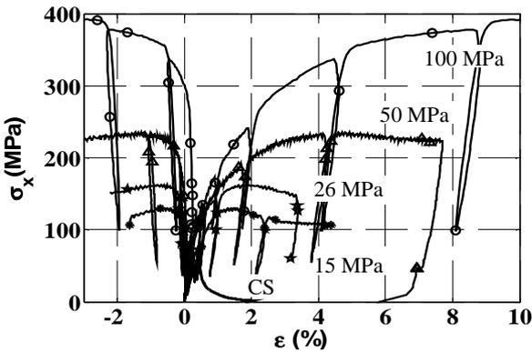
Figure 2: Axial stress vs. axial and circumferential strains for various confining pressures
