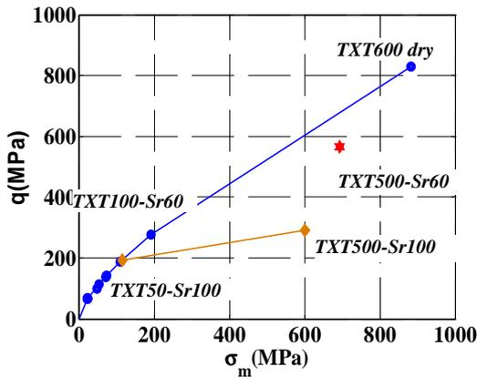
**Figure 6.** Limit states of concrete for the different tests: maximal deviatoric stress vs. mean stress.
