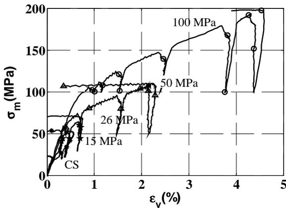
Figure 3. Mean stress vs. volumetric strain for various confining pressures
