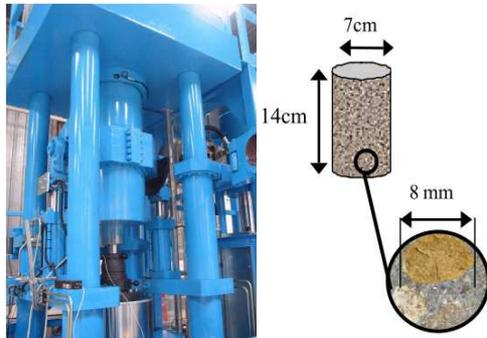
**Figure 1:** GIGA device and specimen dimensions
