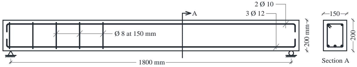
**Figure 2:** Schematic of RC beam
