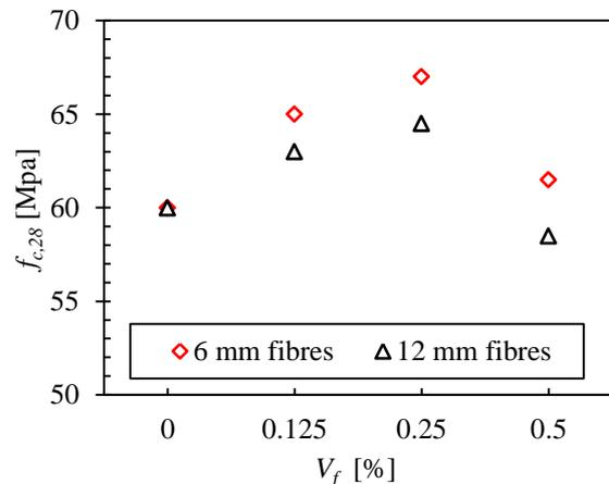
**Figure 3:** 28 days compressive strength of FRCs
