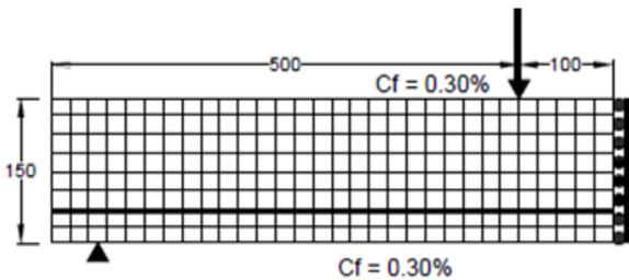
Figure 1: Finite element modeling of the beams.
