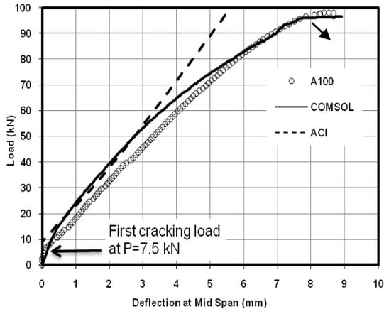
**Figure 2:** Experimental load-mid span deflection curve vs. ACI formula and COMSOL simulation.
