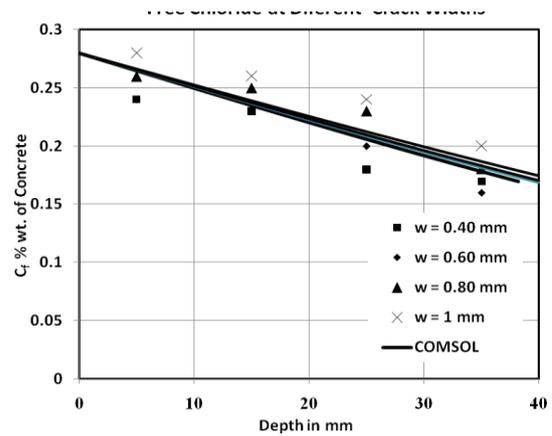
**Figure 4:** Free chloride profile a long crack walls with different crack widths.
