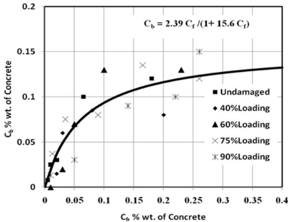
**Figure 3:** Relationship between free and bound chloride.
