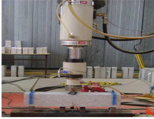
Figure 2: Experimental device of the three-point bending test
