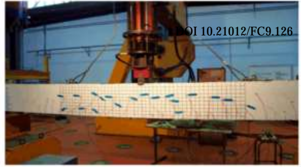
Figure 11 : Experimental test of the beam in the three-point bending
