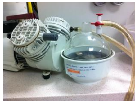
Figure 3. Air-vacuuming of samples after the heating-cooling cycle.
