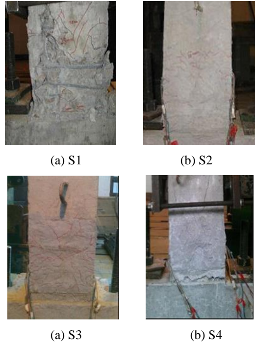
Figure 5: Crack patterns of specimens after failure.
