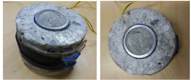
Figure 10: Concrete specimen subjected to a confining pressure of 50 MPa.
