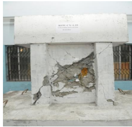
Figure 13: Complete cracking and concrete crushing of web wall and boundary element in RSW-CY-1.25
