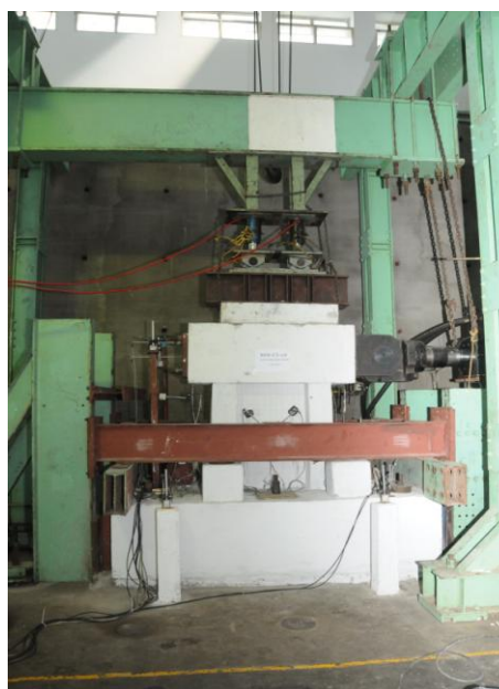
Figure 7: Test set-up of shear wall.
