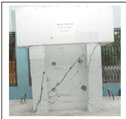
Figure 11: Final cracking pattern in shear wall RSW-MO-1.0.
