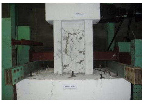
Figure 12: Final failure of shear wall RSW-CY-1.5.
