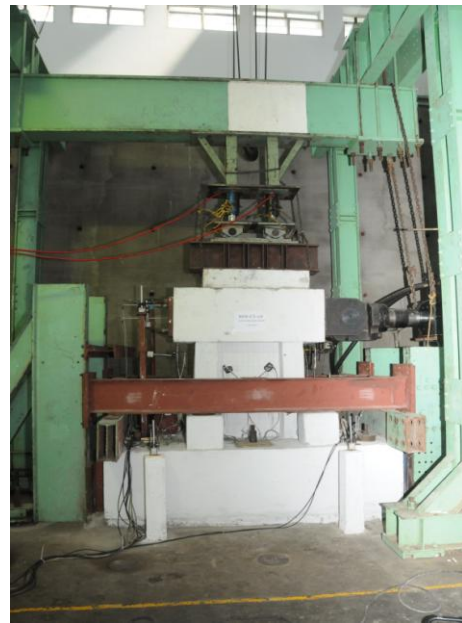
Figure 7: Test set-up of shear wall.
