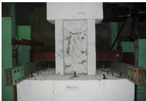
Figure 12: Final failure of shear wall RSW-CY-1.5.
