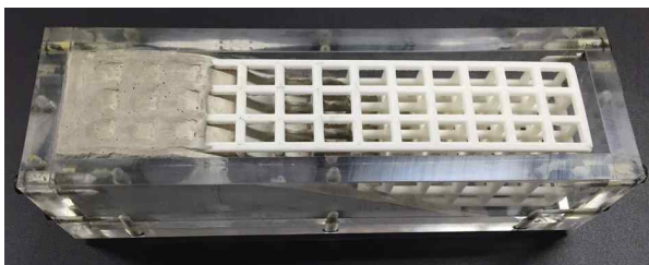
Figure 12: Aligned fiber filled with mortar (casting halted to show the reinforcement)
