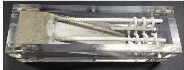
Figure 13: Printed rebar filled with mortar
