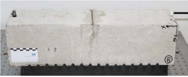
Fig. 9: Determination of the dynamic flexural modulus vibration analysis
