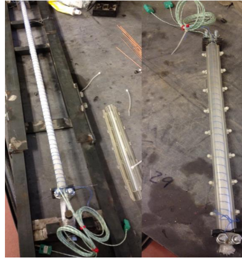
Figure 8: SMP tendon manufacture process left and completed tendon right.
