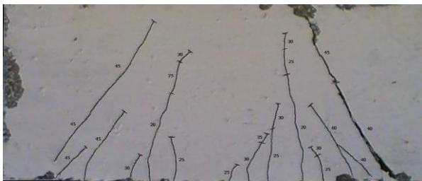
Fig. 16. Crack pattern and mode of failure of the control beam BC1(2Ø12 CFRP) ( P_{cr} = 200 KN and P_{ult} = 450 KN)
