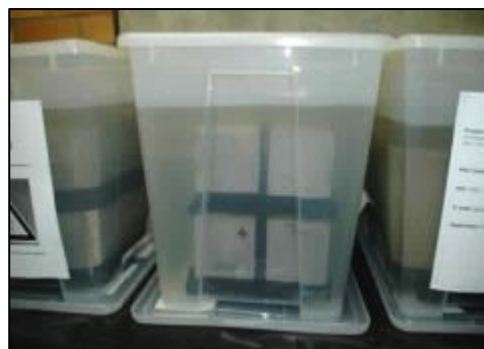
Figure 1 : Immersion of concrete specimens in 7% sulphuric acid solution.
