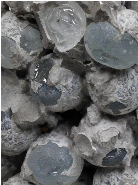
Figure 4: Effect of aggregate surface roughness on post-failure appearance: (a) unroughened surfaces; (b) roughened surfaces
