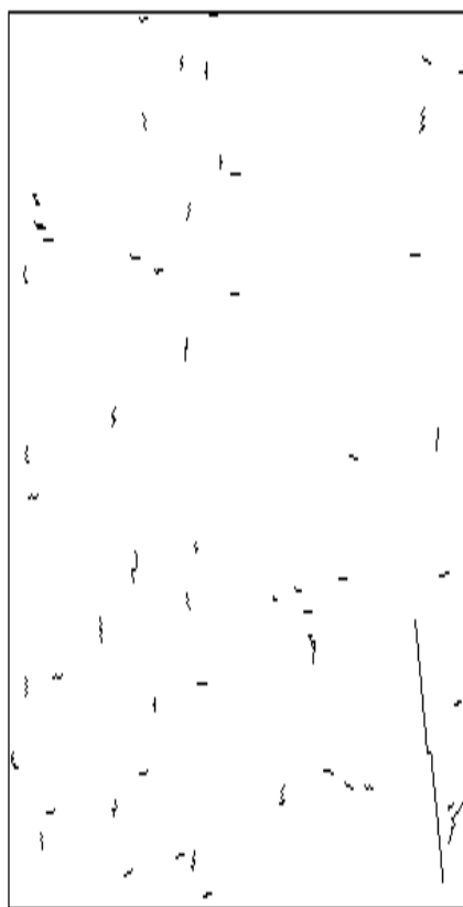
Figure 9 Crack propagation simulation for fully confined condition
