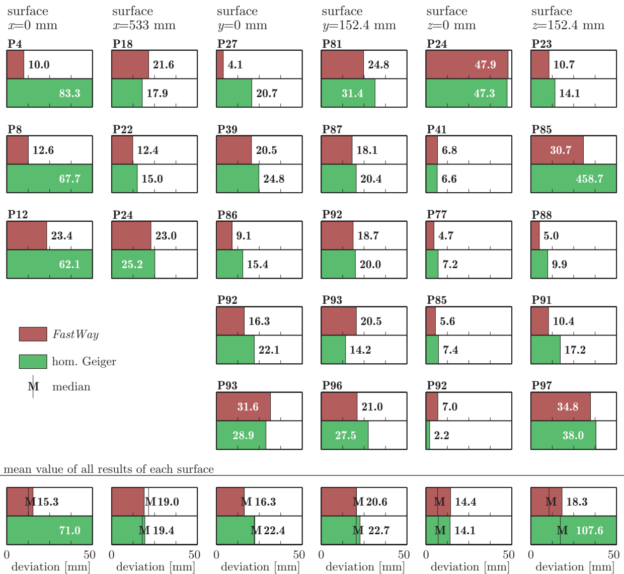
Figure 4: Display of the deviation between the estimated and the actual source locations. In the last row the mean (colored bar) and the median of the deviation computed for each surface separately are shown.
