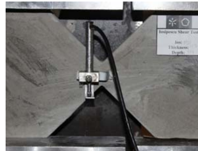
Figure 8: The position of the LVDT to measure the sliding of the shear crack formed in the notched section
