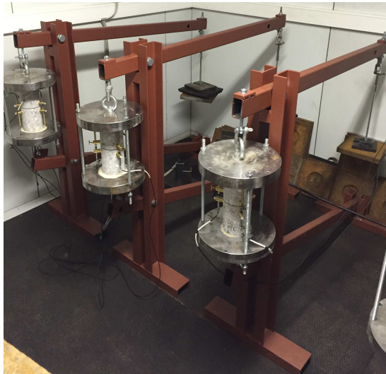
Figure 5: creep frames with specimens during creep test
