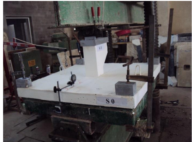
Figure 2 Punching shear test.
