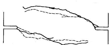
Figure 13: Nooru-Mohamed test: experimental crack pattern for P_s = 10 \text{ kN} .
