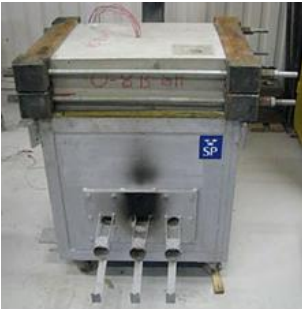
Figure 1: Experimental setup with specimen placed on top of the small-scale furnace [6].
