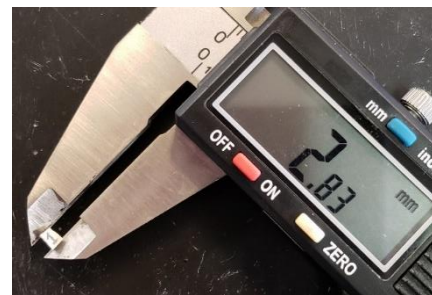
Figure 2 : Final geometry of samples used for ice quantification
