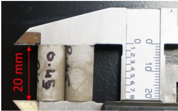
Figure 1: Geometry of the samples used for length change measurements
