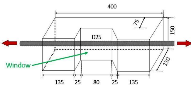
**Figure 3:** Lay-out of the test specimen (units: mm)
