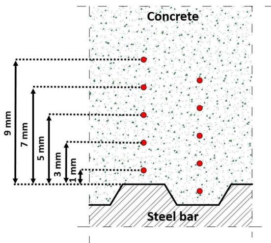
**Figure 10:** Lay-out for two points with different positions (1-3-5-7-9 mm).
