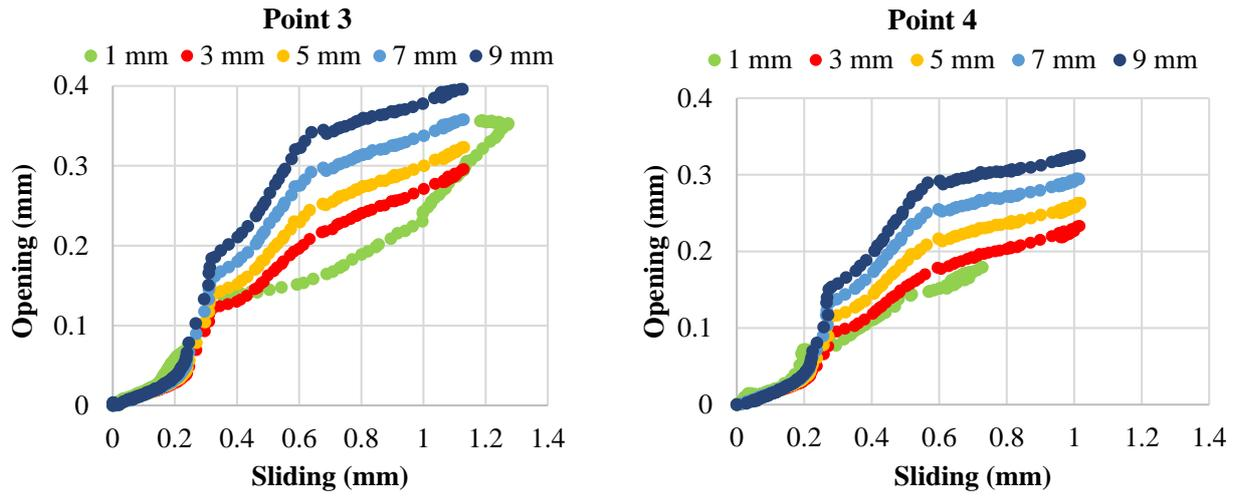
Figure 11: Opening-sliding relationship in concrete for two points at different positions (1-3-5-7-9 mm).
