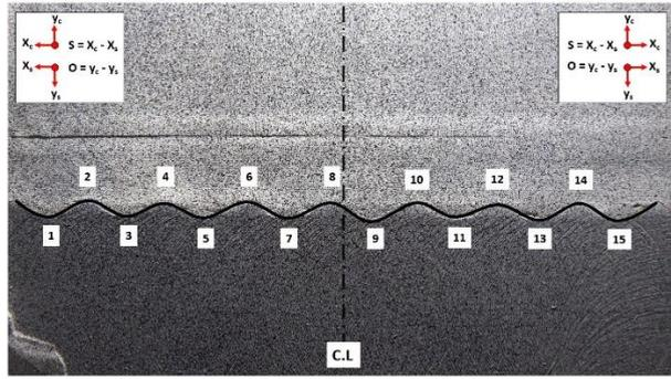
Note:  $S$  is sliding between matrix and rebar,  $O$  is opening between matrix and rebar,  $X_c, Y_c$  are displacements of matrix in X, Y directions respectively,  $X_s, Y_s$  are displacements of rebar in X, Y directions respectively
