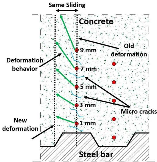
Figure 12: Schematic of opening-sliding behavior in concrete with going vertically from the rebar.
