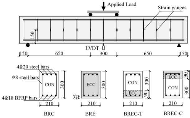
Figure 2: Schematic illustration of test setup and specimen details (mm)
