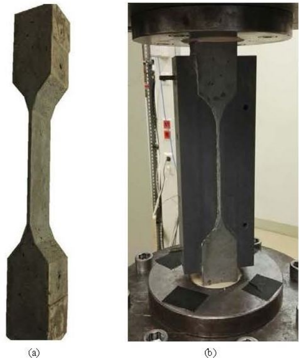
Figure 1: a) Naked unnotched SHCC specimen, b) specimen fixed in the testing machine. The lateral confining elements were removed shortly before load initiation.
