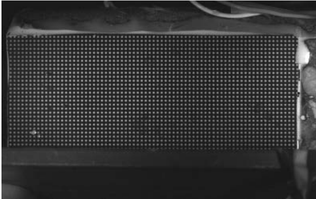
Figure 1: Last recorded frame of a spalling test on HPC concrete with 1 Mfps acquisition speed. (Free-end on the left hand side)
