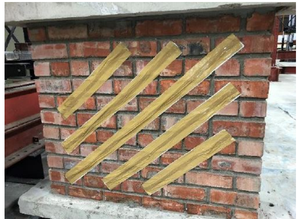
Figure 9: Debonding strips on full scale tests [4]
