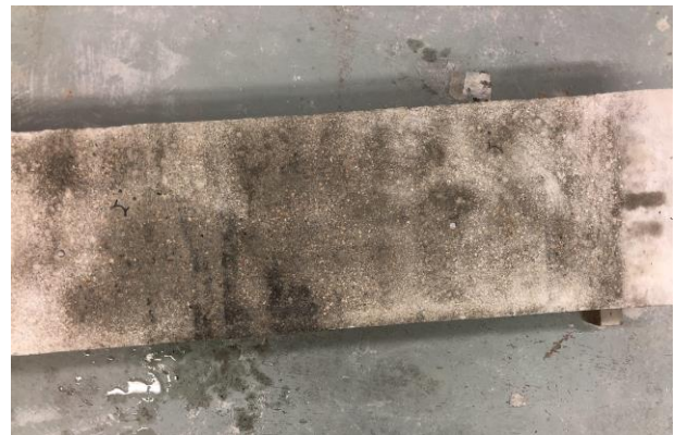
Figure 3: Roughened surface of RC beams
