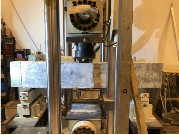
Figure 6: Four-point bending test set-up (S/D=2.5:1)
