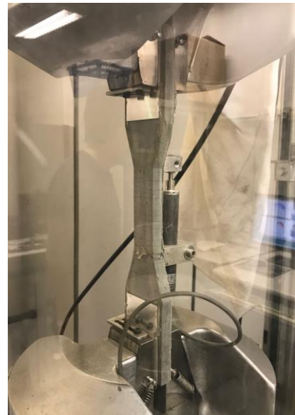
Figure 1: Direct tension test set-up for SHCC
