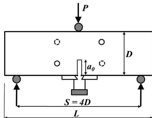
Figure 1: Schematic diagram of test set-up
