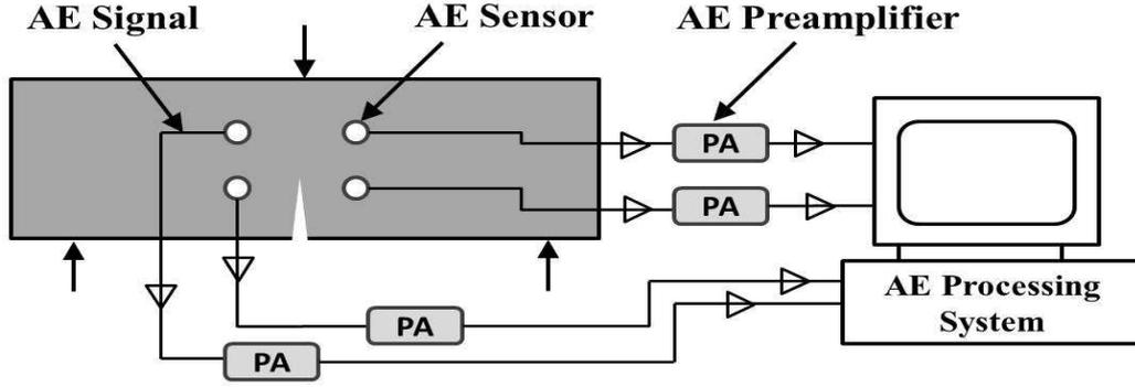
Figure 2: Acoustic emission system schematic diagram
