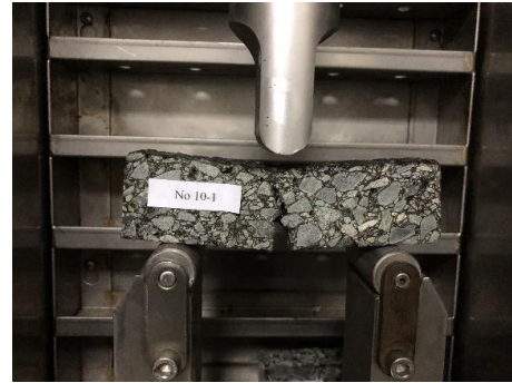
Figure 2: 3-p-b testing system. Temperature was controlled at -10^\circ\text{C} and displacement rate of cross-head was kept at 1mm/min.
