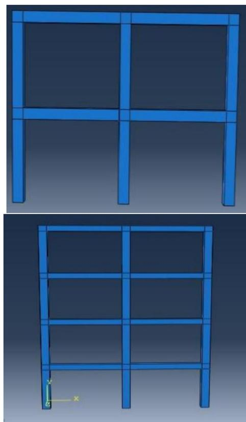
Figure 13: Modeling of two-story and four-story concrete frame
