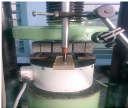
Figure 6. Direct shear test on cement grout beam.
