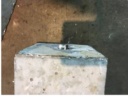
Figure 3: Pullout failure of concrete.
